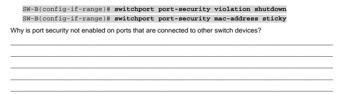
Ports connected to other switch devices have a multitude of MAC addresses learned for that single port. Limiting the number of MAC addresses that can be learned on these ports can significantly impact network functionality.
